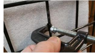
Tighten the Clamp to the desired rod of the grid panel with the Mounting Stud pointed in the direction you want your DragonFly to extend and hand-tighten the clamp. HINT: You won't have to tighten the clamp as much to prevent sagging if you clamp to one of the vertical rods.
